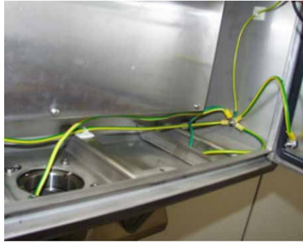
Earthing of the coupling to the housing (Similar to image)
