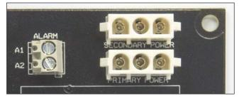
Figure 5.1 - Alarm and Power connections
