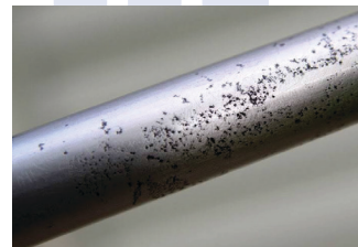
Pitting on Stainless Steel tube after 3 years' service.
