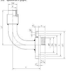
90° quadrant pipe with vibration damper for pressure gauges ≤ NCS 100 (4") only
