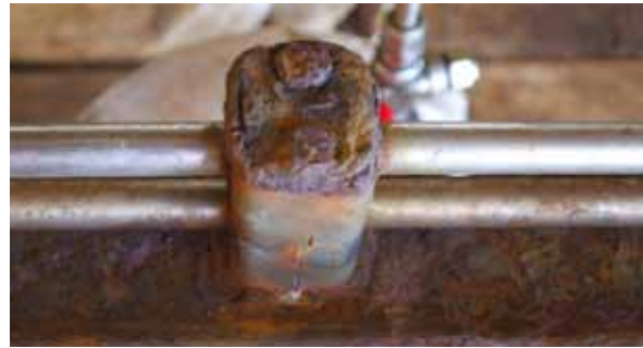
Crevice corrosion between the tube/tube trap interface.
