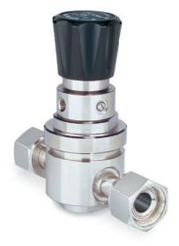
TESCOM 64-3200 Series ultra high purity, high flow tied diaphragm pressure reducing regulator offers 10 R<sub>a</sub> microinch / 0.25 micrometer surface finish and is available in Hastelloy® trim. Maximum flow rates are up to 31.8 SCFM / 900 SLPM, with inlet pressures of 150, 1000, 1500 psig / 10.3, 69.0, 103 bar and outlet pressures up to 200 psig / 13.8 bar.
