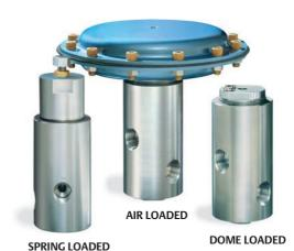
TESCOM 54-2200 Series pressure reducing regulator is designed for high flow and high pressure hydraulic applications. Inlet and outlet pressure is rated up to 8000 psig / 552 bar with  $C_V = 2.0$  for flows up to 60 GPM / 127 LPM. Spring, air and dome loaded versions are available. Hardened Stainless Steel seat and poppet delivers excellent wear resistance.
