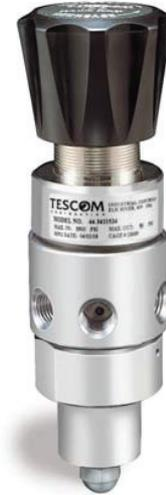
TESCOM 44-3400 Series is a compact, lightweight high purity two-stage cylinder regulator for specialty, corrosive and pyrophoric gases less than 5 SCFM / 141 SLPM. Diffusion-resistant metal-to-metal diaphragm seal ensures gas purity and integrity.
