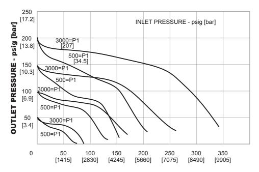
FLOW RATE - SCFM [SLPM] Air C<sub>V</sub> = 1.0
