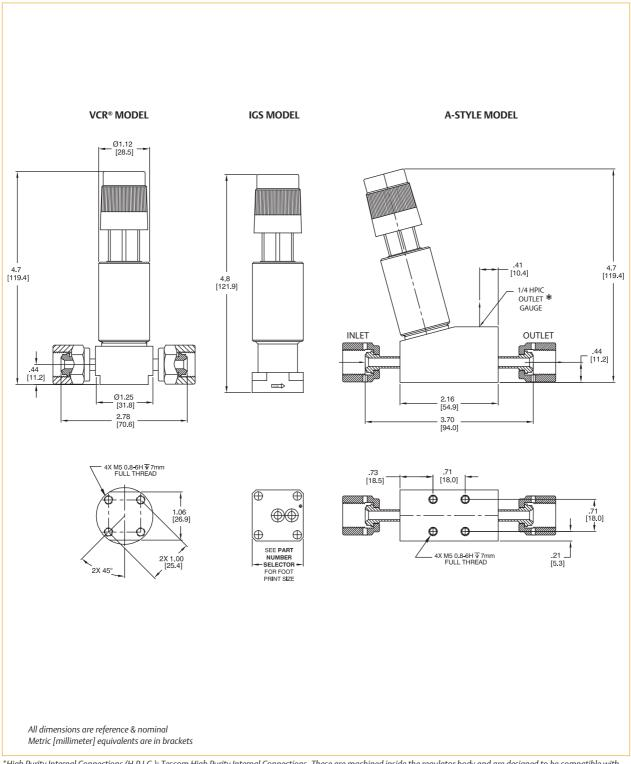
\*High Purity Internal Connections (H.P.I.C.): Tescom High Purity Internal Connections. These are machined inside the regulator body and are designed to be compatible with VCR<sup>®</sup> (or equivalent) male fittings - swivel only.
