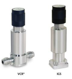
TESCOM 12 Series is a miniature ultra high purity IGS/VCR pressure reducing regulator. The 12 Series offers 5  $R_a$  or 10  $R_a$  microinch finishes, tied diaphragm and internally springless and threadless design. It provides inlet pressures of 150 psig / 10.3 bar, outlet pressure from 250 mm Hg-15, 30, 60, 100 psig / 250 mm Hg-1.0, 2.1, 4.1, 6.9 bar with flow rates up to 120 SLPM.
